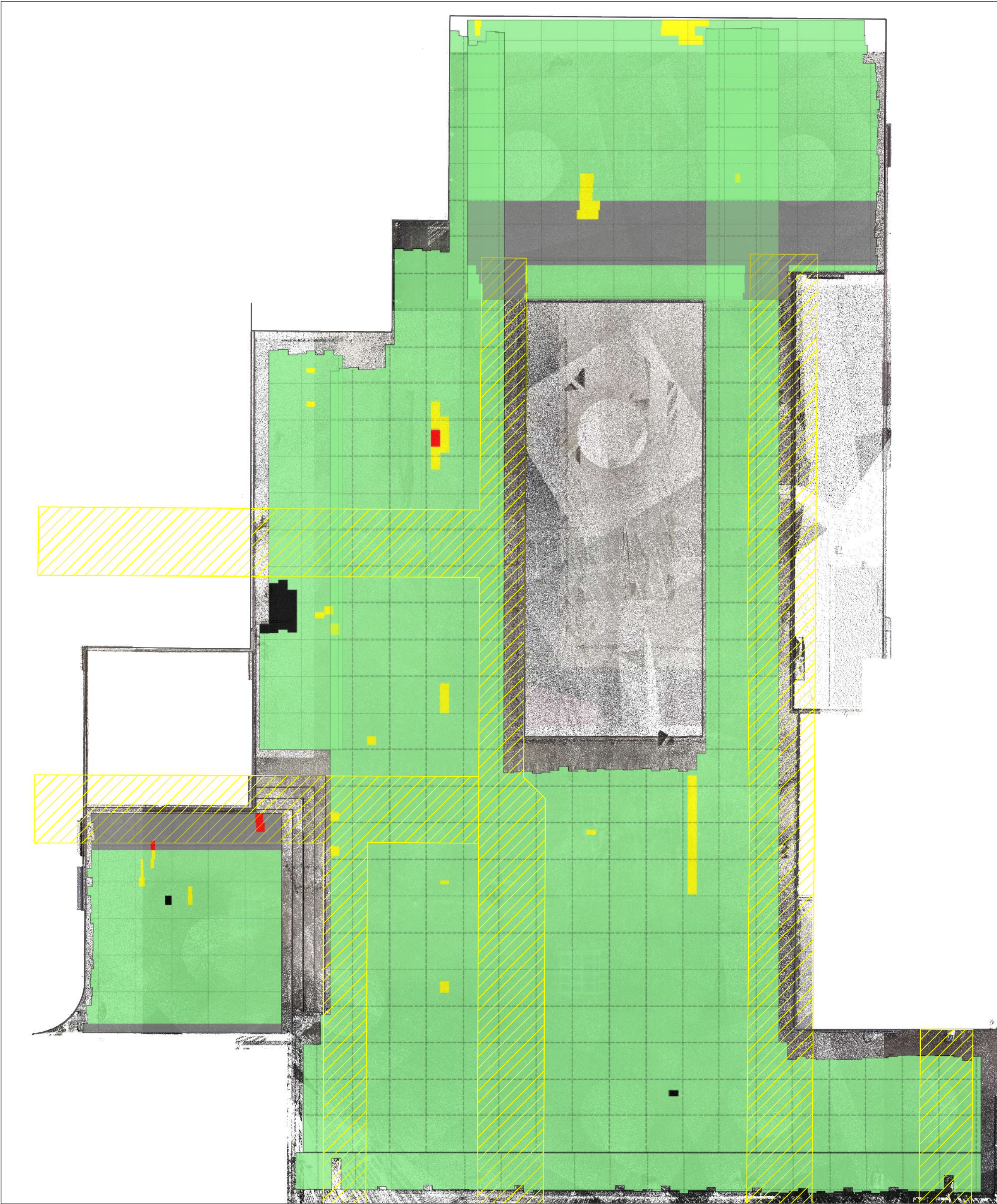
AREA 1 - GPR CORROSION RESULTS- TOP REBAR MAT SCALE: 1:80
